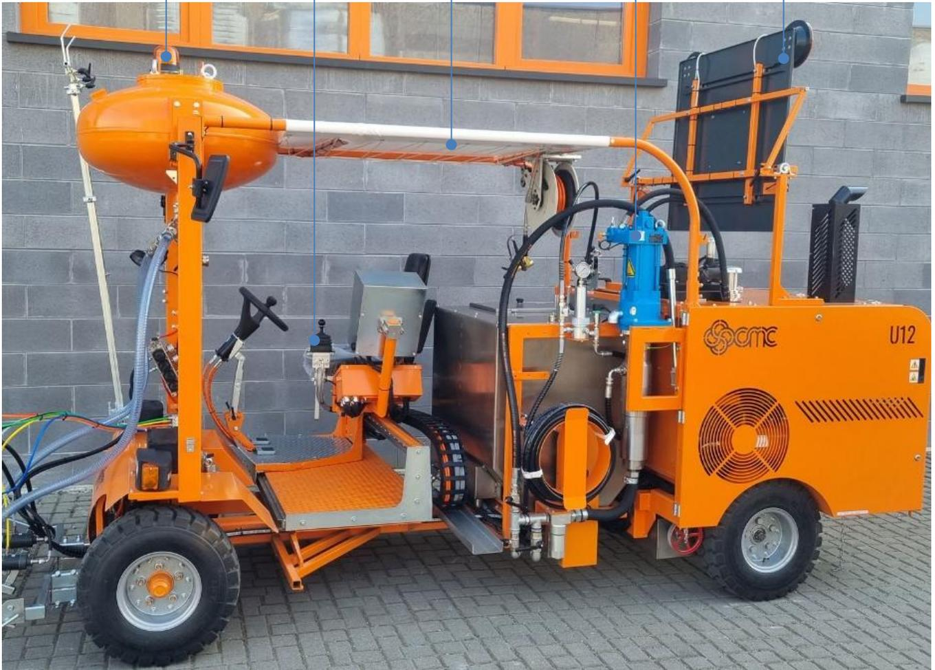
Seats and console unit **sliding** (left/right) up to above marking unit *only with hydraulic steering*
