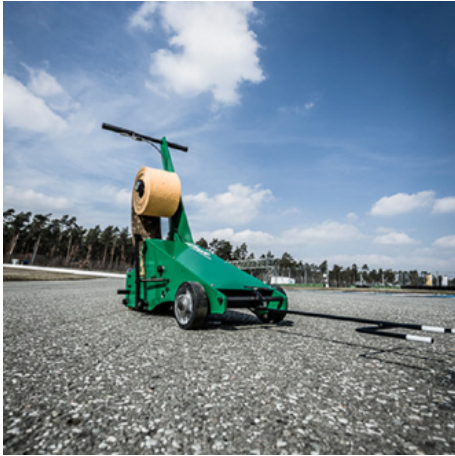
Foil laying technology
