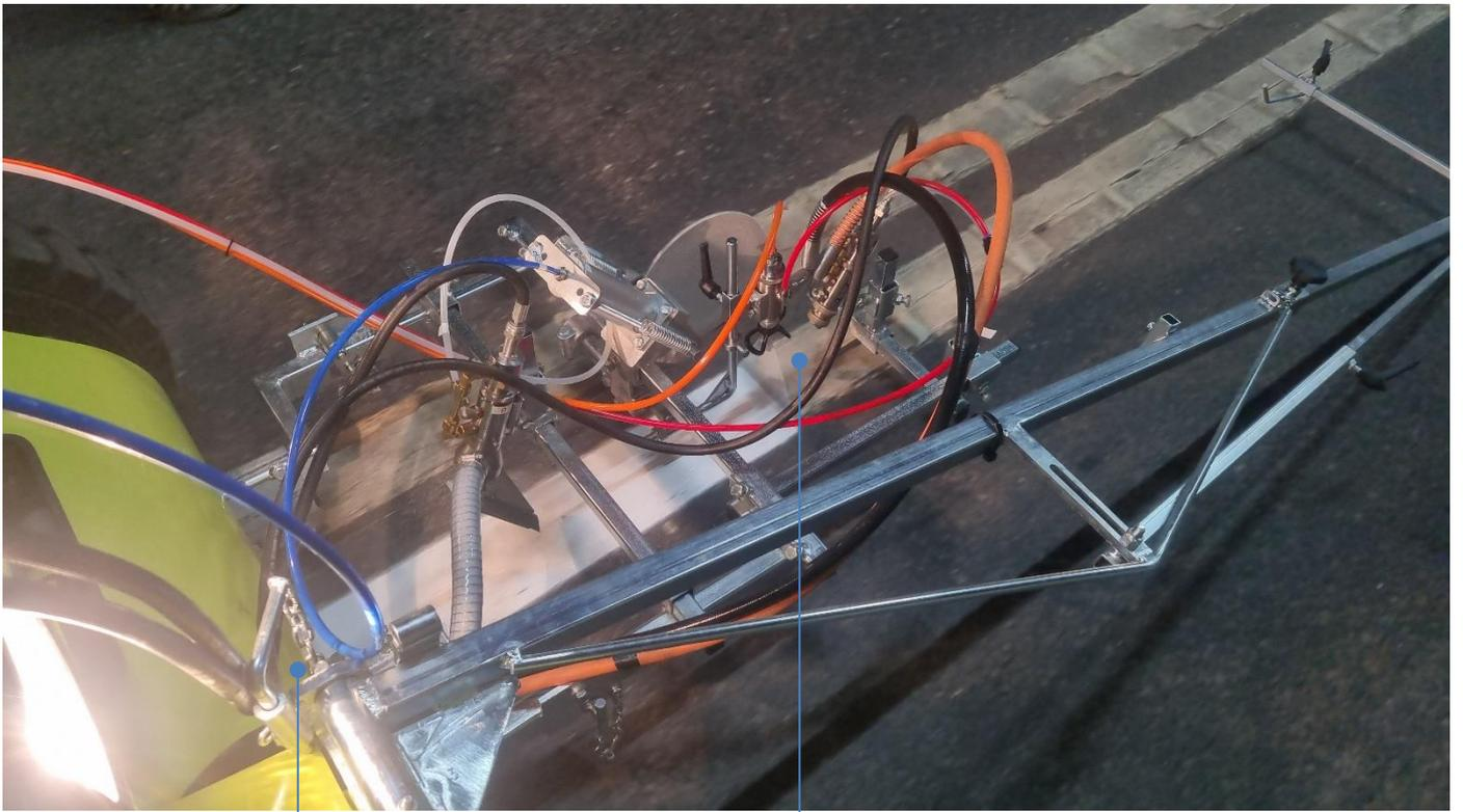
Centrally-mounted marking unit to make the central line with comfort
