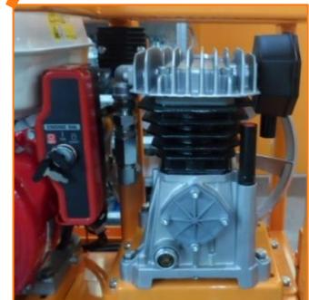
Compressor 255 l/min to supply air to pneumatic controls, to pressurized glass bead tank (optional) and to glass bead gun (optional)
